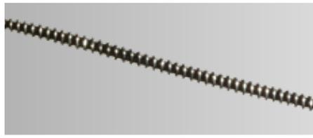
cutting wire - PU flexible foam
