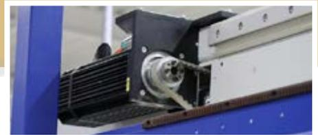
exchange servomotor knife turning unit
