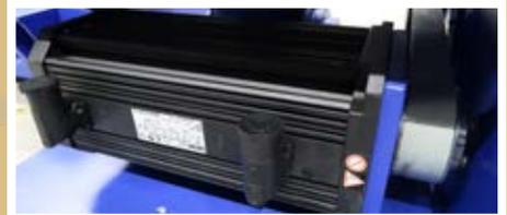
exchange servomotor height adjustment
