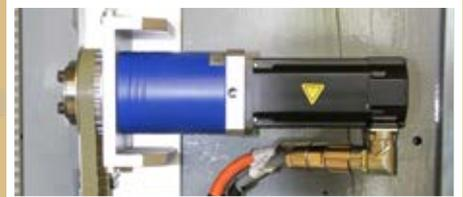
exchange servomotor knife turning unit
