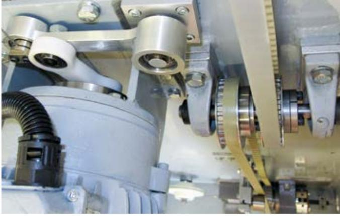
exchange of spare parts oscillation drive
