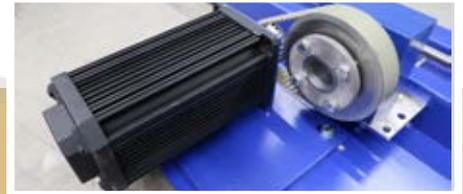
exchange servomotor table drive
