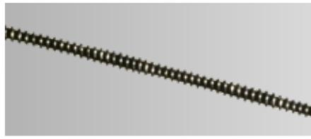
cutting wire - PU flexible foam
