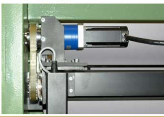
exchange servomotor rollers of holding down device
